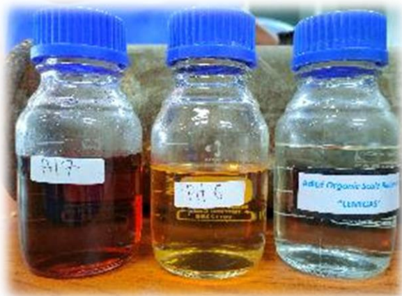
Hasil Sintesis Aditif Organik Scale Removal Variasi pH
