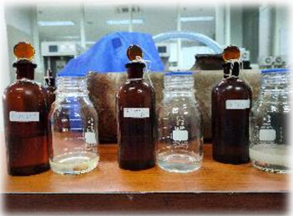
Uji Coba Kereaktifan 1% Aditif (HCl; H 2 SO 4 ; P-TSA)
