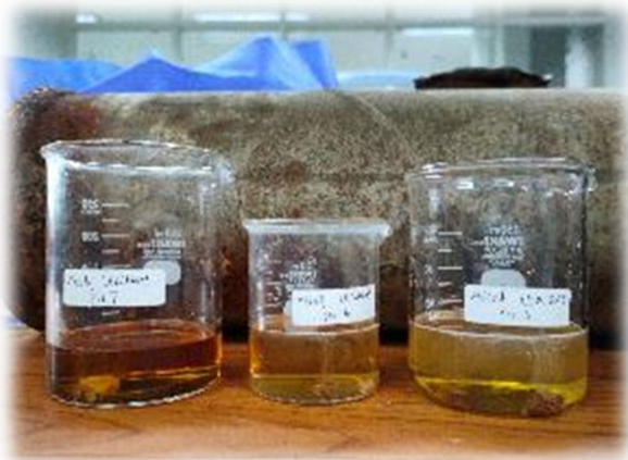
Uji Coba Kereaktifan Aditif Organic Scale Removal (pH : 7;6;5)
