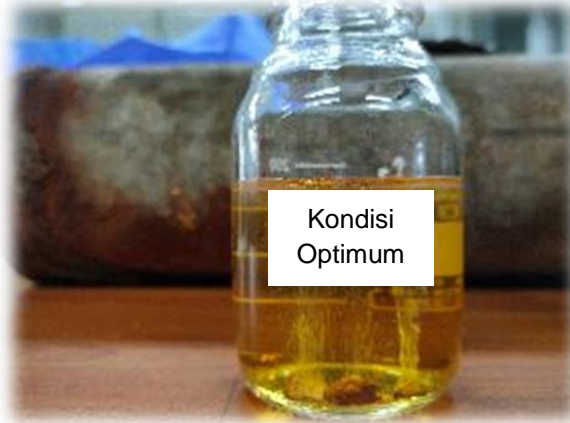
Uji Coba Kereaktifan Aditif Organic Scale Removal hasil upscaling 20 liter
